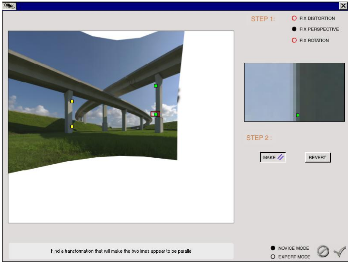
Figure 17: Correcting slight perspective and rotation errors using the Andromeda LensDoc plug-in.
